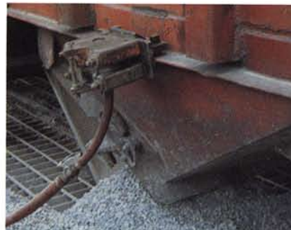
Model SVC-8000 mounted on side to remove coal.
