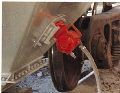
Model CCW-5000 used for removing chemicals from R.R. hopper car.
