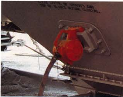
Model CCW-5000 removing PVC powder.
