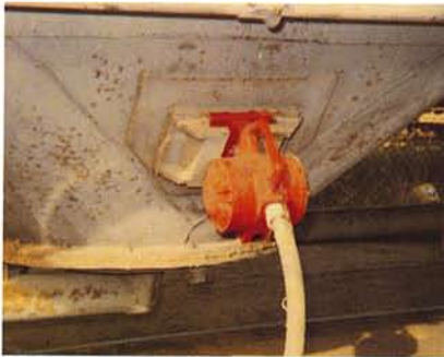
Model CCW-5000 used on R.R. hopper storage car containing sawdust.
